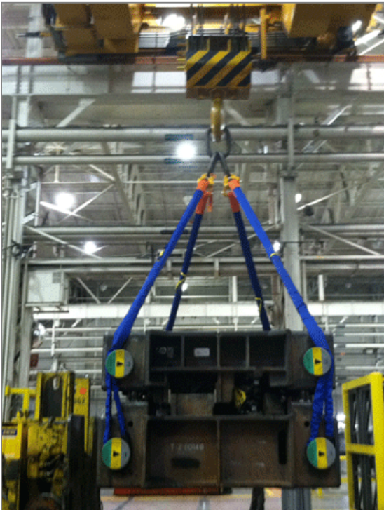
master assemblies to fit crane hooks
